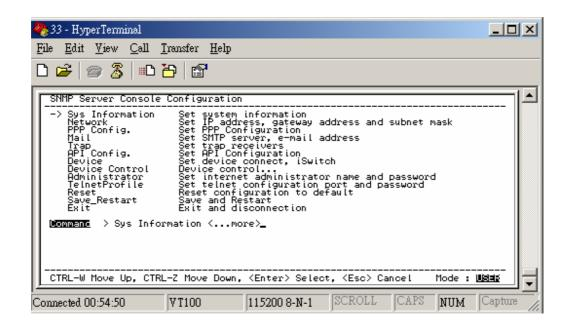
14. Ctrl-Z moves the cursor down and Ctrl-W moves the cursor up. Pick Network, then hit enter.
